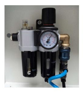
Picture 6.4: Air Lubricator Unit
