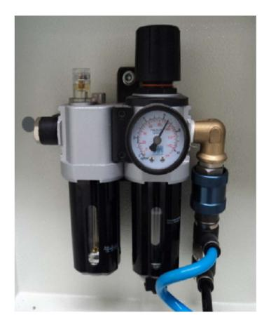
Picture 8.2: Air Lubricator (Lubrication)
