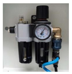
Picture 7.1: Air Lubrication Unit
