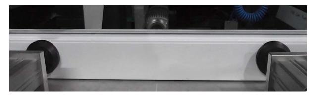
There are 2 clamping pistons on the machine to perform operations on aluminum and PVC profiles. The machine will not start unless the profile is fixed.
