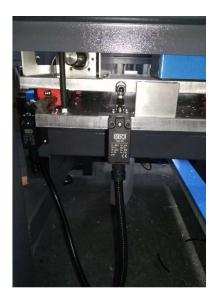
There are mechanical switches at the reference points of the 3 axes of the machine. When any situation is encountered, when the machine is sent to the reference from the screen, the machine will go to its original position, that is, to the zero point. If the axis passes the mechanical switch when it is moved by manual control. Mechanical Stoppers, whose zero point is out of bounds, will stop the axis.
